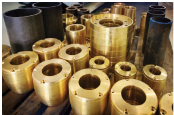
Completed propeller-end housing and thrust housing parts fill a pallet at Seatorque Control Systems.
