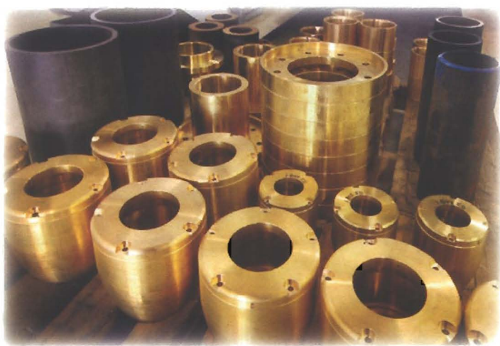
Completed propeller-end housing and thrust housing parts fill a pallet at Seatorque Control Systems.
