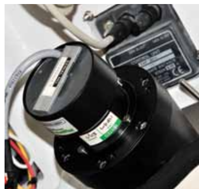
Operation of the electronic helm, seen here from under the console, is precise, effortless and reliable. Long hydraulic plumbing runs are replaced by easy-to-install wiring, and the likelihood of hydraulic leaks are virtually eliminated.
