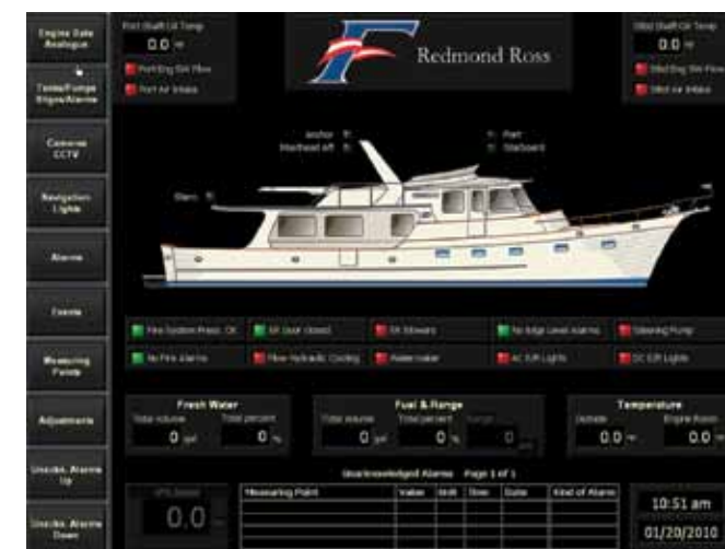
The MAIN PAGE shows all yacht systems at a glance and is used like an aircraft's pre-flight checklist.
