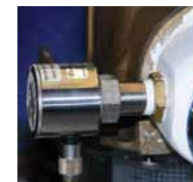
Individual sensors monitor a wide variety of systems and conditions. Here, a vacuum sensor measures restriction caused by a buildup of debris or fouling in a raw water intake. This will alert the captain to a problem long before reduced water flow becomes critical.
