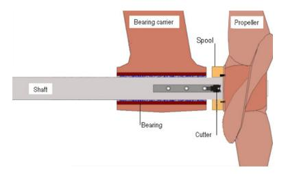
The QuicKutter<sup>TM</sup> is fixed to the bearing carrier and protrudes out over the Quickwater spool surface ensuring that the clearance does not allow rope or line to pass under the blade and that rope or line is continually cut away to allow a continuous flow of water to exit from the bearing.
