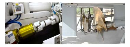
The Seatorque Enclosed Shaft System is a self-contained, oil-filled shaft and thrust bearing assembly designed to increase horsepower, fuel economy and engine life while minimizing shaft noise and vibration. The system is supplied as a single unit from the propeller end to the engine input coupling accommodating any length shaft and diameters up to seven inches.
