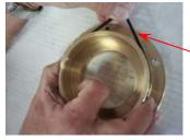
4) To Remove and replace the o-rings on the outside nose of the seal carrier (step 8, page 4) place the index finger and thumb on opposite sides of the carrier nose and squeeze upwards stretching the ring. With the other hand pull the O-ring out of the groove and discard.
