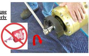
NOTE: DO NOT USE LOCTITETM WHEN INSTALLING THE SHAFT COUPLING BOLT.
