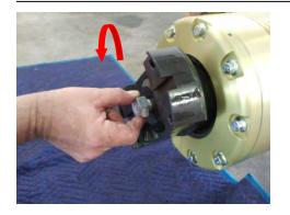
3) Remove the Bolt in the center of the shaft coupling.
