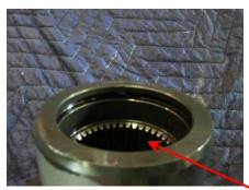
19) Lubricate the internal and external splines of coupling and shaft with Seatorque shaft oil.
