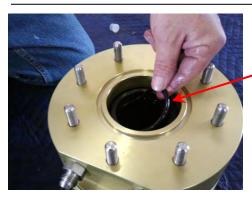
15) **Check point**; Make sure the Oil Impeller O-ring seal is installed in the groove provided inside the bore of the bearing housing as shown.
