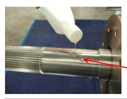
16) Pre-oil spline and shoulder of shaft thoroughly with Shaft Oil; also making sure that the bore of the Thrust housing and O-ring are well lubricated.
