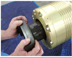
5) Remove all nuts & washers holding the thrust housing in place on the Isolator Mount Bolting Flange. Slide the thrust housing assembly off the end of the splined shaft. Wrap the housing in a protective cover and place in a clean area until required, the thrust bearings are inside the housing and therefore attention to cleanliness is imperative.
