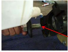
21) Lubricate the threads of the Main Coupling Bolt with shaft oil and install Shaft Bolt and Coupling Washer to end of shaft. Hand tighten bolt until it is snug against the coupling.
