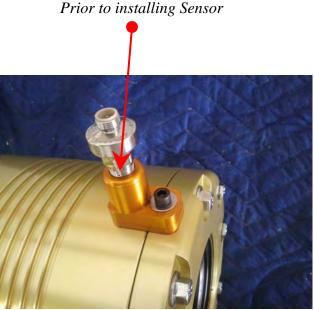
Half Fill Sensor Port with Shaft Oil
