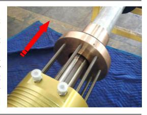
18) **Check point**, Make sure that the coupling O-ring is installed in the groove provided inside the
