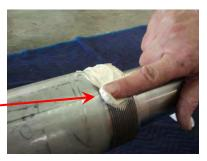
**Note:** Casing has a machined nose with flat face finish designed to mate with a seat in the isolator Housing providing a positive seal when tightened, an O-ring is also included to ensure a permanent seal. The 5200 is necessary to seal threads against water intrusion and possible crevice corrosion.
