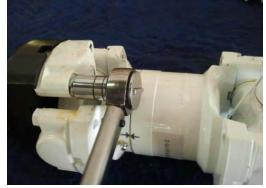
minimum ½" inside of the total slip available for the installation to be correct. Should conditions exceed this specification please contact Seatorque Factory for help and assistance.
